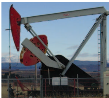
Figure 1 Pump jacks are found over oil wells in many parts of Alberta. This one is near Cochrane, Alberta.
